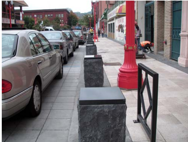
Figure 12 – Festival bike rack and street light pole protected by bollards
